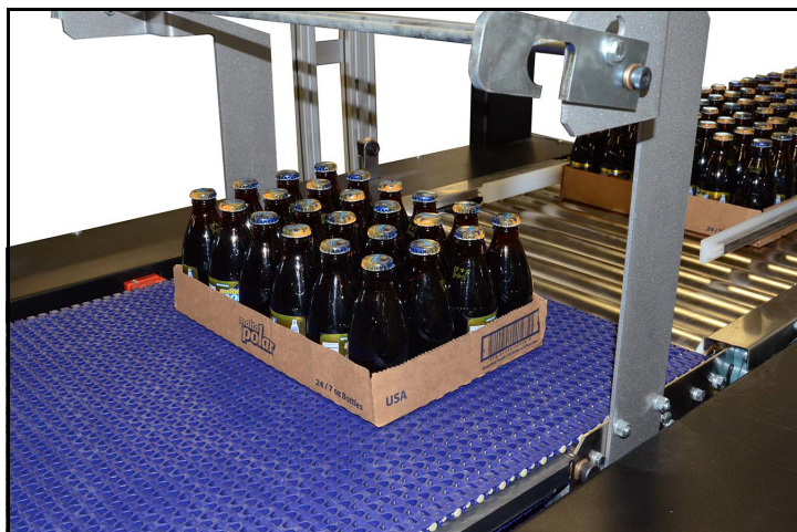
Figure 2-4 - In-feed to Acceleration Conveyor
